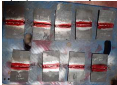
Gambar 6. Proses Pengujian NDT Liquid Penetran
