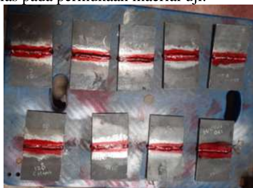
Gambar 6. Proses Pengujian NDT Liquid Penetrant
