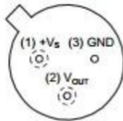
NDV Package 3-Pin TO-CAN (Top View)
