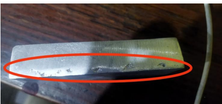
Gambar 22. Cacat Lubang Gas (650°C, 700°C, 750°C)
