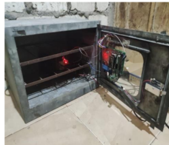
Gambar 5. Rancangan Prototype Sistem Proteksi OLT
