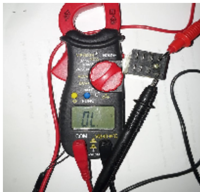
Gambar IV.10 Hasil Pengujian Coil Relay
