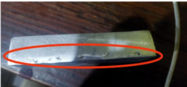
Gambar 22. Cacat Lubang Gas (650°C, 700°C, 750°C)
