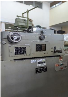
Gambar 9. Proses uji keausan Ogoshi
