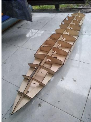
Rangka bodi drone
