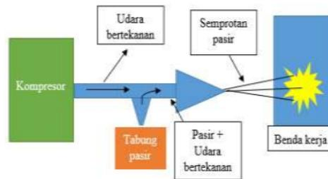
Gambar 3. Proses sandblasting
