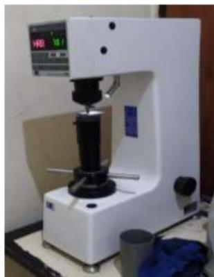
Gambar 8. Rockwell Hardness Tester
