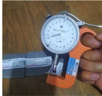
Gambar 4 Elcometer 122 Testex® Replica Tape
