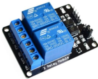
Gambar 2. Modul relay 2 kanal.
