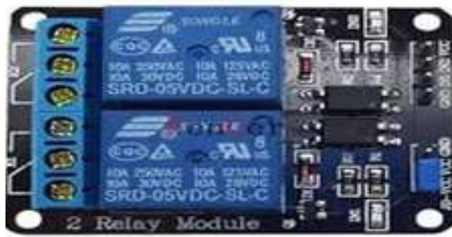
Gambar 6.1 modul relay 5v
