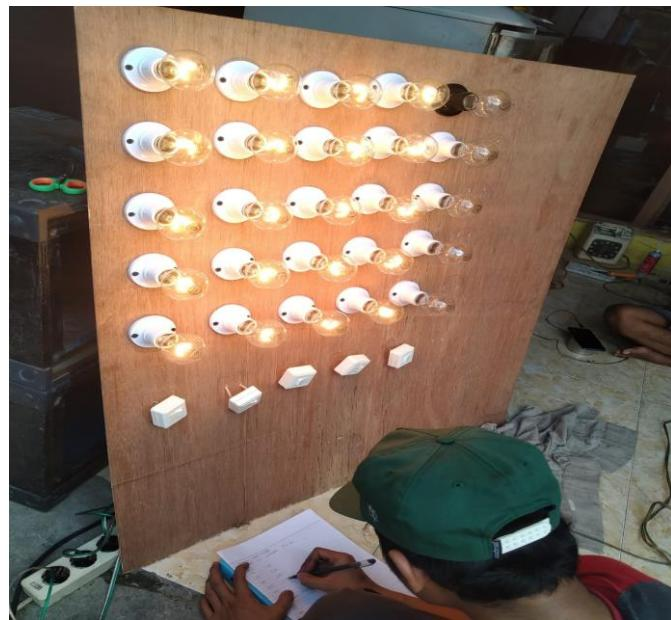
*Gambar 5 Pemebebana bohlam lampu*
