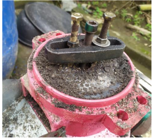
Proses pencopotan molding
