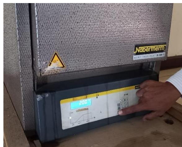
Gambar 4. Pre Heating 200°C
