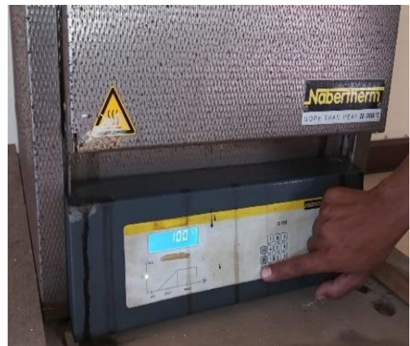
Gambar 3. Pre Heating 100°C
