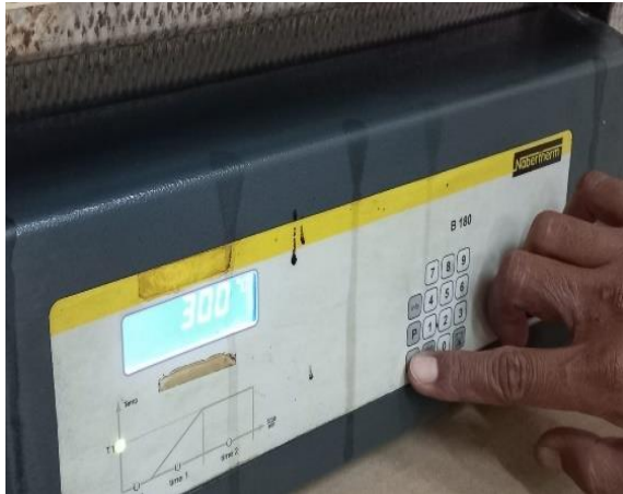
Gambar 5. Pre Heating 300°C
