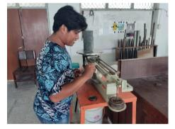
2. After weighing the wet weight of the concrete, the concrete is put into the oven at a predetermined temperature for ± 24 hours. After being baked, the concrete is removed from the oven and weighed to determine the dry weight of the concrete to determine the absorption results obtained.
