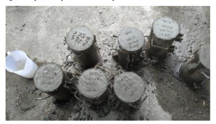
2. After that, weigh the wet volume weight where the wet weight is the weight of the cylinder plus the weight of the concrete in the cylinder. After weighing the wet volume, then 1 day after weighing the wet volume weight, the concrete is removed from the mold and will be curing.
