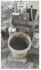
4. The process of weighing water and superplasticizer according to the calculation of the mix design. The planned water-cement ratio to be used is 0.3 in accordance with the f'c plan. For superplasticizer is used in the casting process to be carried out using a percentage of 0.4% by weight of cement.
