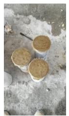
2. The next step is to test the compressive strength of concrete for 7 days, 14 days and 28 days in order to determine the strength value of the concrete that is given a load. With this concrete compressive strength test, you can also find out whether the designed concrete can meet the design compressive strength or not.
