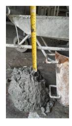
2. The next stage is that the concrete mixture is inserted into each of the cylinders that have been provided, then after entering 1/3 part, knead the mixture so that the concrete can be evenly distributed to the surface, also do 2/3 parts, and finally 3/3 parts. Then fill again until it fills the surface of the cylinder. Don't forget to leveling the surface of the concrete with a trowel so that the surface can be flat and neat.
