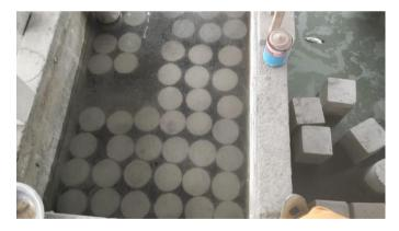
4. After lifting the curring pool, 1 day after the concrete is removed from the curring pool, the dry volume weight will be weighed in order to determine the difference between the concrete before it is immersed in the curring pool and after being removed from the curring.
