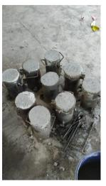
3. After being removed from the mold, the concrete is put into the curing pond so that the concrete does not lose water quickly and also to maintain the temperature of the concrete to be cured. Curing was carried out for 6 days, 13 days, and 27 days a day before the compressive strength test was carried out.
