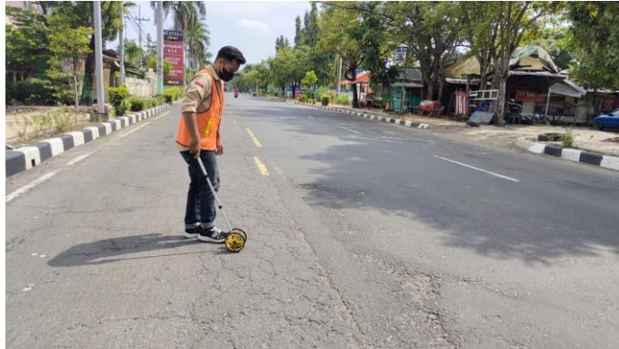
Figure A 10 Calculation Area of Crocodile Cracking (Source : Reseacher Data, 2022)
