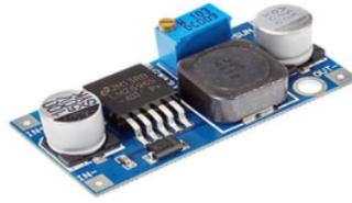
Gambar 2.1 Modul Step down LM 2596
