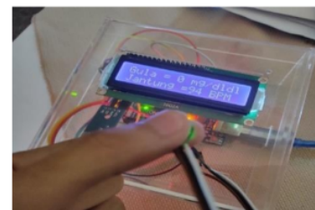
Gambar 3.1. Uji sensor TCRT5000 dan Pulse Sensor SEN11574
