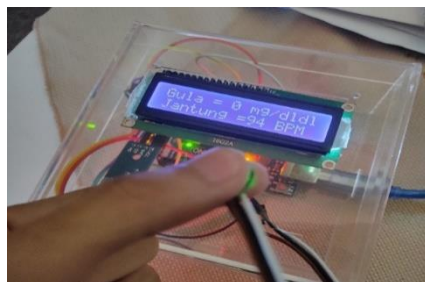
Gambar 3.1. Uji sensor TCRT5000 dan Pulse Sensor SEN11574
