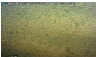
Gambar 4. 29 (c) Gambar struktur mikro anoda larutan NaCl 5%
