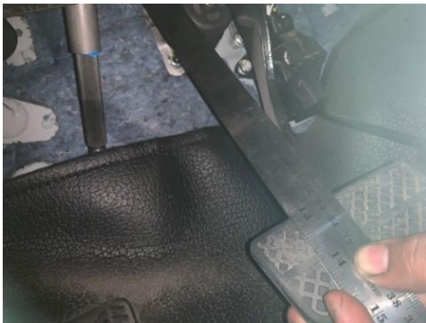
Jarak Pedal Pushroad 34 cm = 0.34 m
