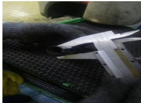
Diameter master rem 18 mm = 0.018 m
