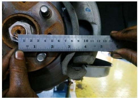
Diameter Radius Efektif Piringan Rem 9.5 cm = 0.095 m
