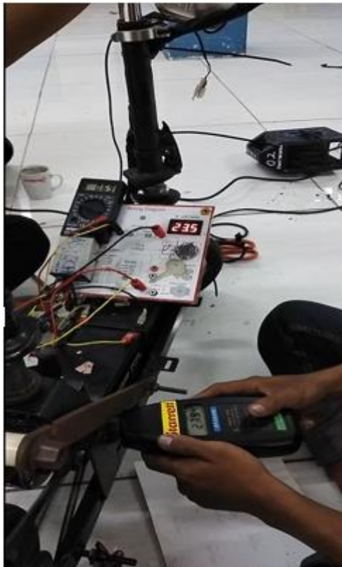
pengujian alternator diameter 65mm Rpm 2700
