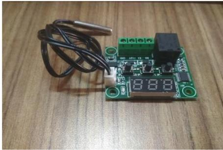
**Gambar 2.13** PCB Rangkaian Sensor Suhu (thermostat)
