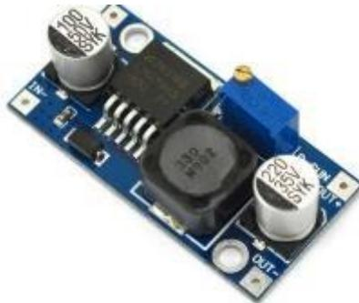
**Gambar 2.7 LM2596 DC-DC Step Down**
