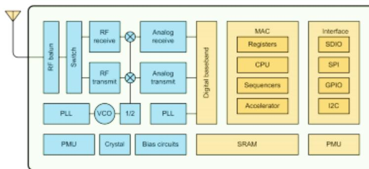
Figure 1 ESP8266EX Block Diagram
