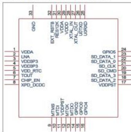
Figure 2 Pin Assignments
