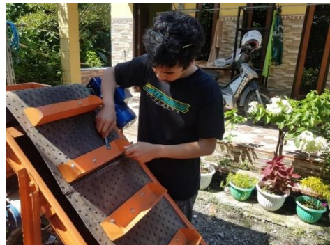
Memasang Bucket Conveyor
