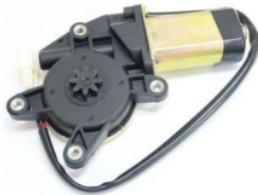
Gambar 2. 7 Motor dc *power window*
