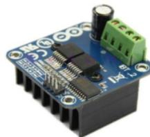
Gambar 2. 8 Driver motor bts7960
