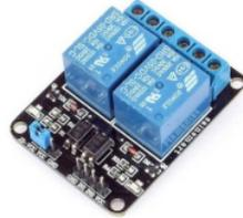
Gambar 2. 4 Relay 2 channel
