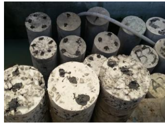
Proses perendaman beton
