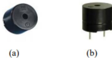
Gambar 2. 5 (a) Buzzer tampak atas (b) Buzzer tampak samping
