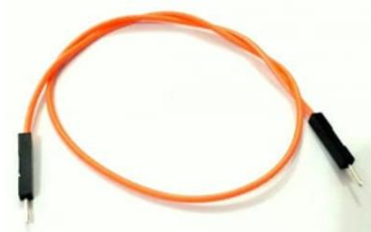
Gambar 2.12 gambaran kabel jumper male to male
