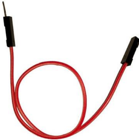
Gambar 2.13 gambaran kabel jumper male to female
