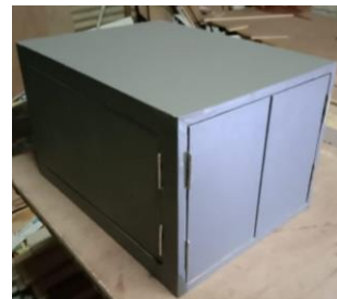
Gambar 4.1 Prototype pintu truck box
