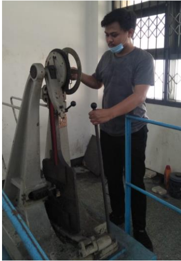
Pengujian impact di LAB material Untag surabaya
